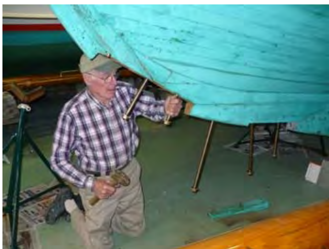
Jarvis Newman of Southwest Harbor, Maine, who pioneered making Friendship sloops out of fiberglass, works in his shop to restore an original wooden Friendship christened Old Baldy. The vessel was used to create a mold for the first Newman fiberglass sloops.
