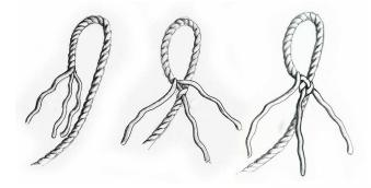
Untwisting the strands of the standing part of the line, holding the strands open, and pulling through a strand to form each step of a splice, while keeping the yarns of the strands from catching on each other, are operations that all need to happen at almost the same time.
