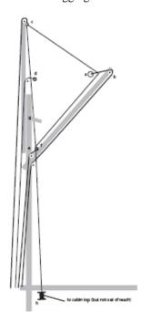
(b) and halyard blocks (c) were the same. Even our block on the gaff jaws (e) to "tweak the shape" made a great in-haul for the new roller-cable. Now this line just ties loosely to the roller cable (f). The inhaul line (d) of the sail needed minor adjustments, but basically worked just fine also. I'm always happy to not have to drill through good varnish if I don't have too. We did have to buy a larger roller spool (h) and a bit of new lightweight dacron line.
